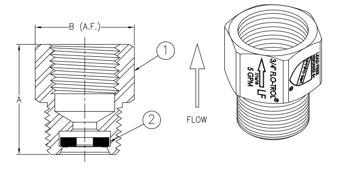
Max Temp 180°F (82°C) Max Pressure 125psi (8.6 bar)
