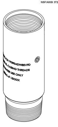
Max Temp 200°F (93°C) Max Pressure 4400psi (303bar)
