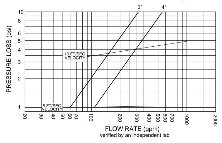
Note: For longer service life & higher efficiencies it is not recommended that flow velocities exceed 10 feet/second
