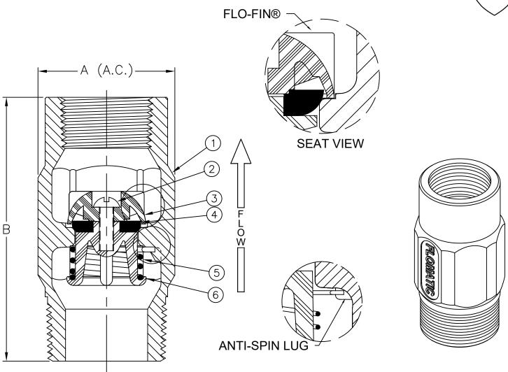
Max Temp 180°F (82°C) Max Pressure 400psi (28bar)
