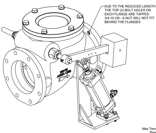
Max Temp 180°F (82°C) Max Pressure 250psi (18bar)
