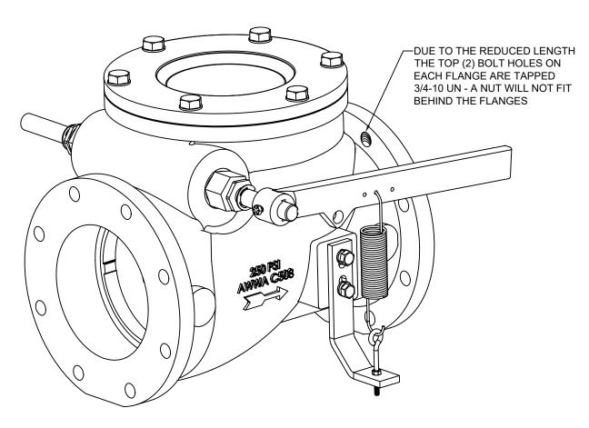
Max Temp 180°F (82°C) Max Pressure 250psi (18bar)
