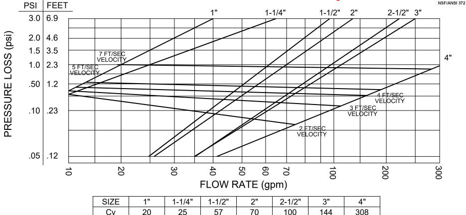
Note: For longer service life & higher efficiencies it is recommended that flow velocity be between 2 to 4 feet/second
