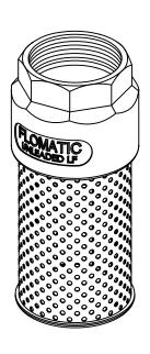
Max Temp 180°F (82°C) Max Pressure 250psi (18bar)
