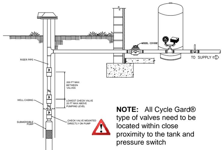
**NOTE:** All Cycle Gard® type of valves need to be located within close proximity to the tank and pressure switch
