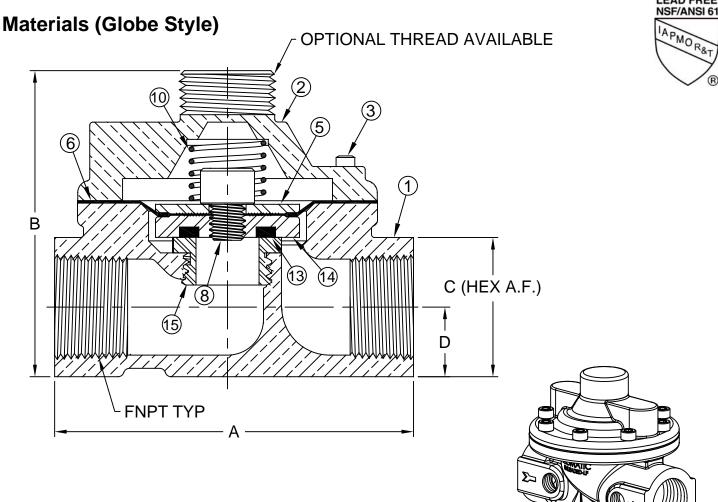
Max Temp 180°F (82°C) Max Pressure 400psi (28bar)
