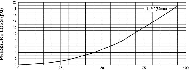
FLOW RATE (gpm) VALVES TESTED FULLY OPEN WITH NO SPRING
