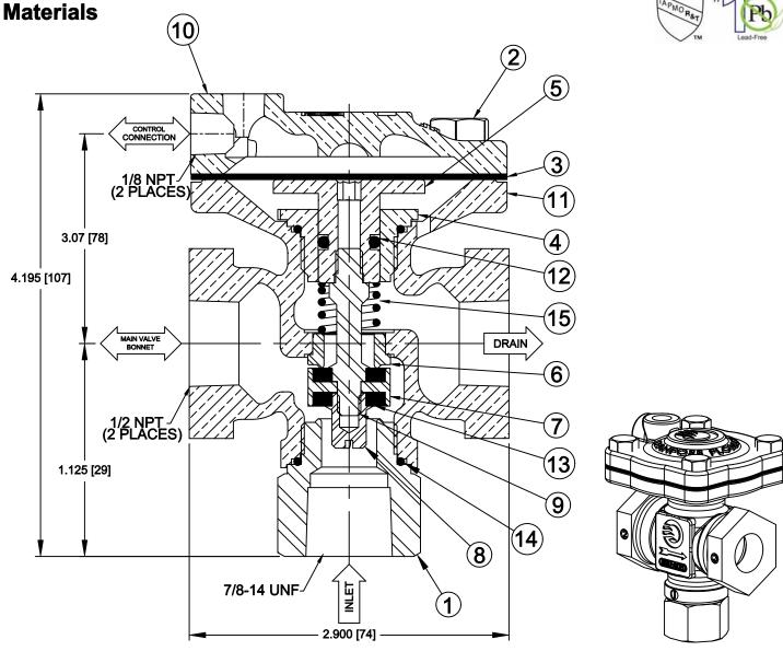
Max Temp 180°F (82°C) Max Pressure 300psi (21bar) Weight 2.1 (.95)
