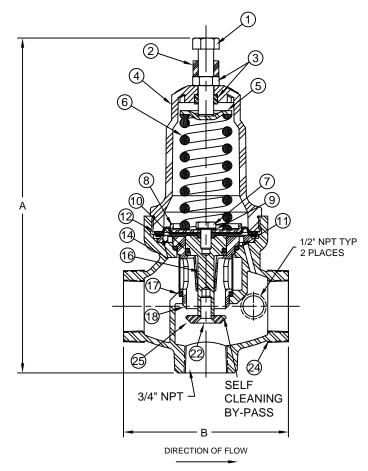
Max Temp: 180°F (82°C) Max Inlet Pressure 400psi (27bar)
