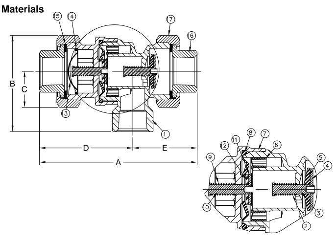
Max Temp 210°F (98°C) Max Pressure 175psi (12bar)
