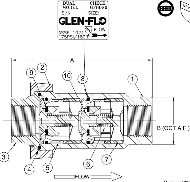
Max Temp 180°F (82°C) Max Pressure 175psi (12bar)
