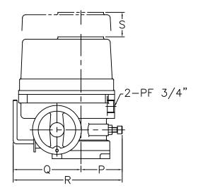
**NOTE:** When installing an actuator, proper clearance around the actuator is required to ensure that the cover can be removed to allow for maintenance. Refer to dimension "S".
