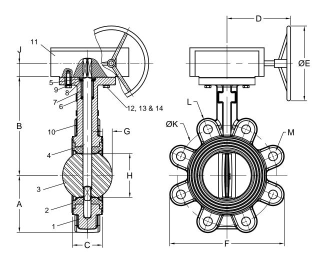
Max Temp 220°F (104°C) Max Pressure 250psi (17bar) Bi-Directional & Dead End Service Pressure Rating 250psi (17 bar)
