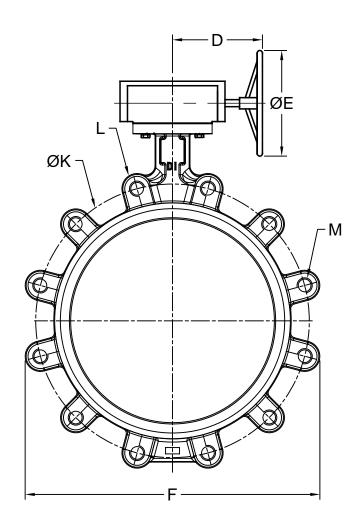
Max Temp 220°F (104°C) Max Pressure 250psi (17bar) Bi-Directional & Dead End Service Pressure Rating 250psi (17 bar)
