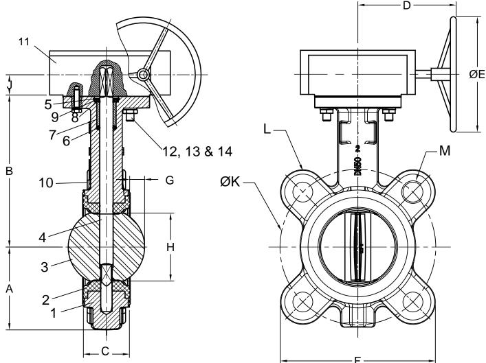
Max Temp 220°F (104°C) Max Pressure 250psi (17bar) Bi-Directional & Dead End Service Pressure Rating 250psi (17 bar)
