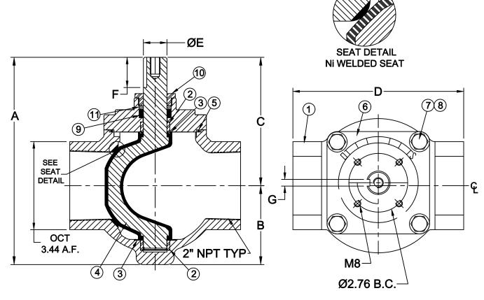
Max Temp 180°F (82°C) Max Pressure 200 psi (14 bar)
