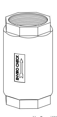
Max Temp 180°F (82°C) Max Pressure 400psi (28bar)
