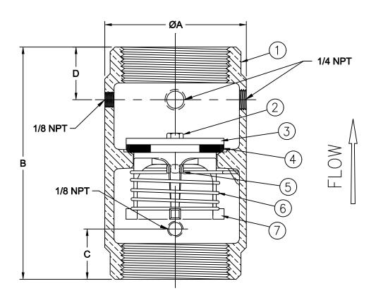
Temp Max: 180°F (82°C) Pressure Max: 400 psi (28 bar)
