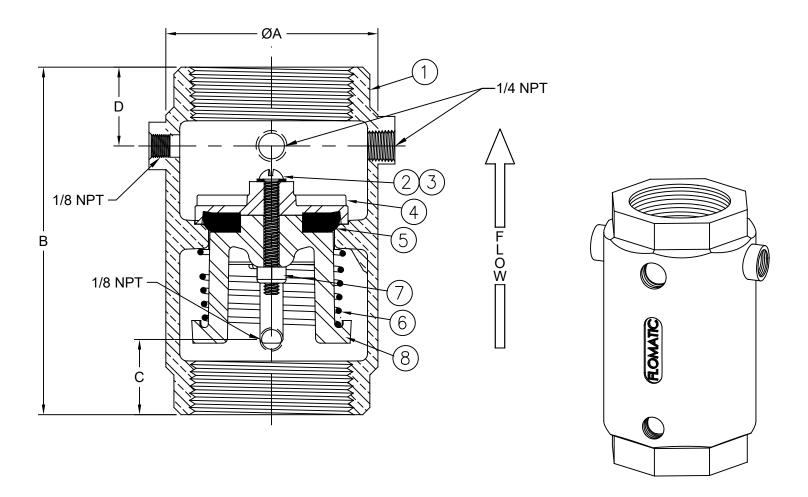
Temp Max: 180°F (82°C) Pressure Max: 400 psi (28 bar)
