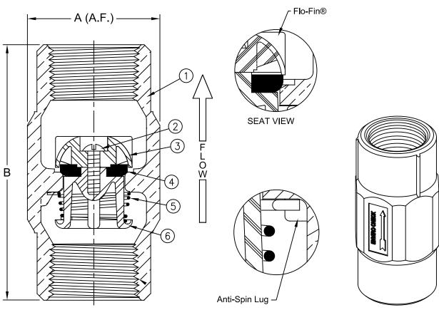
Temp Max: 180°F (82°C) Pressure Max: 400 psi (28bar)
