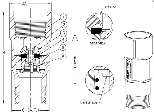
Temp Max: 180°F (82°C) Pressure Max: 400 psi (28bar)
