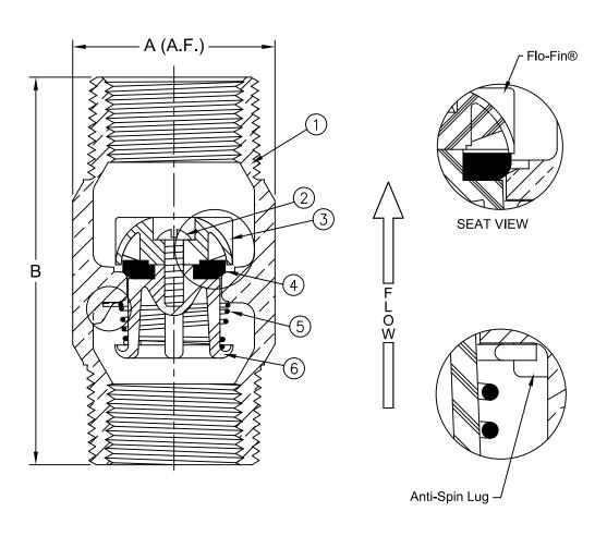
Max Temp 180°F (82°C) Max Pressure 400psi (28bar)
