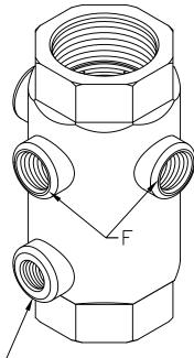
Max Temp 180°F (82°C) Max Pressure 400 psi (28bar)
