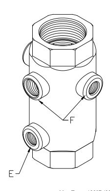
Max Temp 180°F (82°C) Max Pressure 400 psi (28bar)
