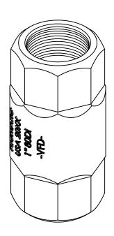
Max Temp 180°F (82°C) Max Pressure 600psi (41bar)
