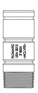
Max Temp 180°F (82°C) Max Pressure 600psi (42bar)
