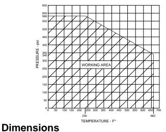
Max Temp 662°F (350°C) Max Pressure 580psi (40bar)
