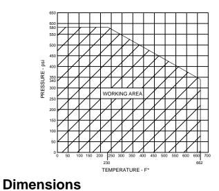
Max Temp 662°F (350°C) Max Pressure 580psi (40bar)
