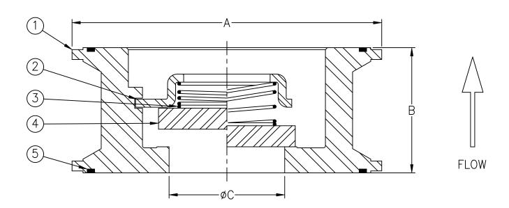
Max Temp 450°F (232°C) Max Pressure 1000psi (69bar)
