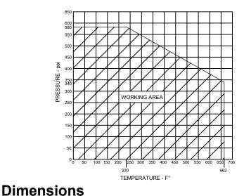
Max Temp 662°F (350°C) Max Pressure 580psi (40bar)
