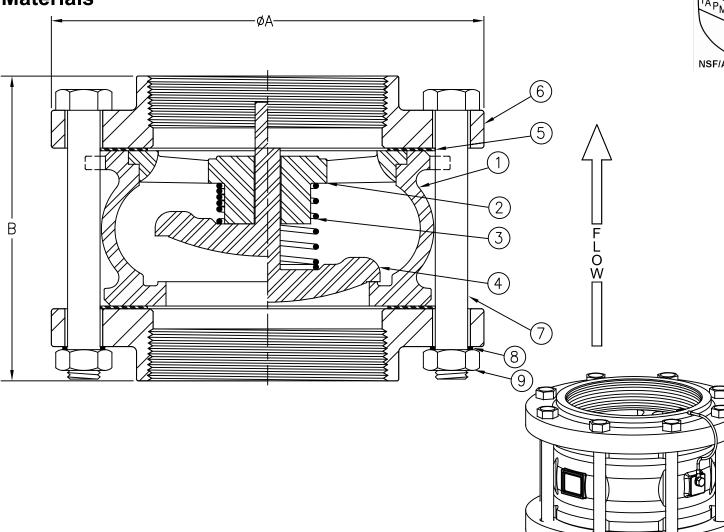
Max Temp 400°F (200°C) Max Pressure 300psi (21bar)
