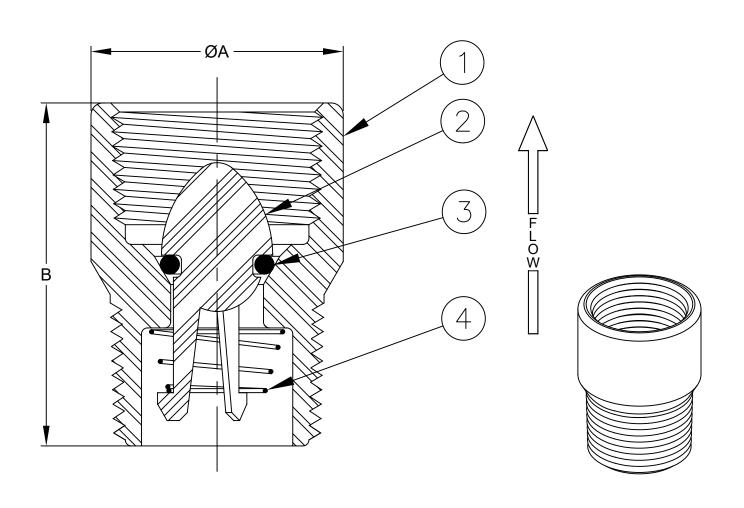
Max Temp 180°F (80°C) Max Pressure 400psi (28bar)
