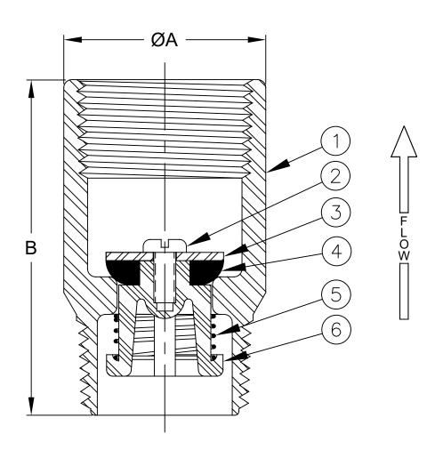
Max Temp 180°F (80°C) Max Pressure 400psi (28bar)
