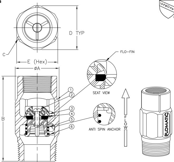
Max Temp 180°F (82°C) Max Pressure 400psi (28bar)
