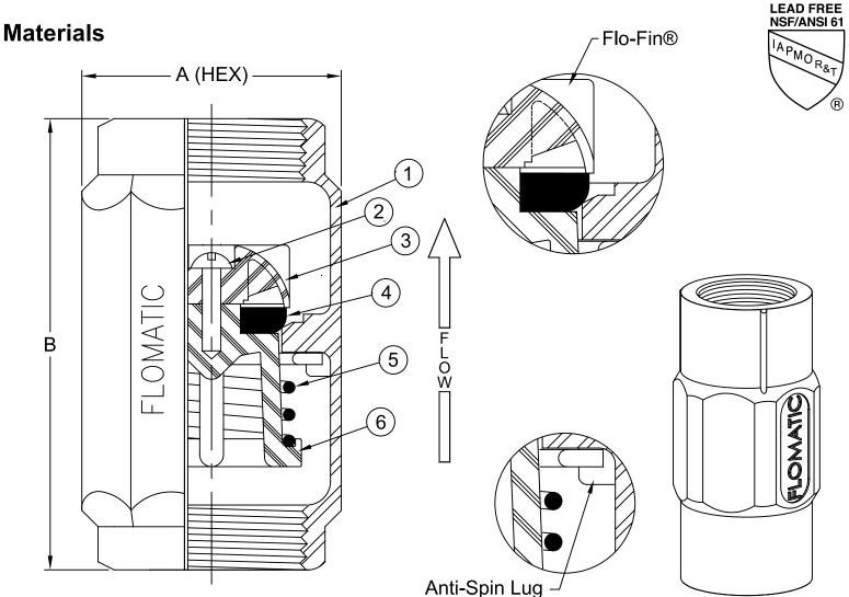
Temp Max: 180°F (80°C) Pressure Max: 400 psi (28 Bar)
