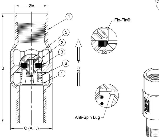
Max Temp 180°F (82°C) Max Pressure 400psi (28bar)
