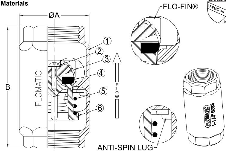
Temp Max: 180°F (80°C) Pressure Max: 400 psi (28 Bar)
