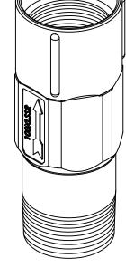
Max Temp 180°F (82°C) Max Pressure 400psi (28bar)
