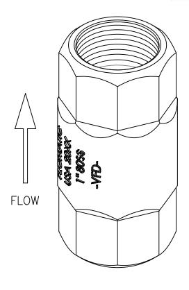
Max Temp 180°F (82°C) Max Pressure 450psi (31bar)
