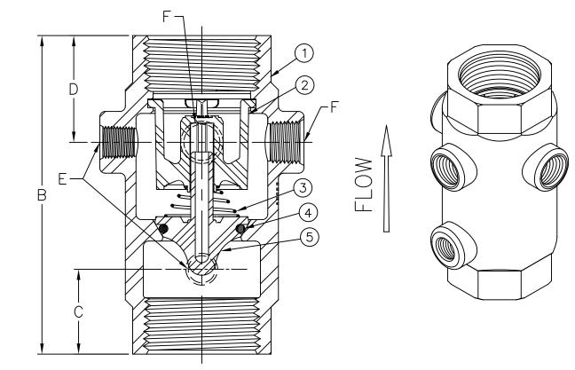
Max Temp 180°F (82°C) Max Pressure 400 psi (28bar)
