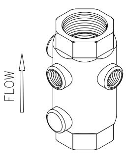
Max Temp 180°F (82°C) Max Pressure 400 psi (28bar)
