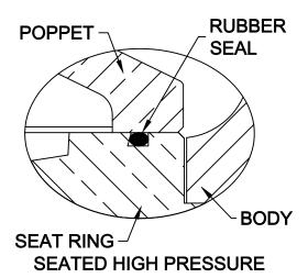
PROVIDES DRIP-TIGHT SEATING AT LOW PRESSURES WITHOUT DAMAGE TO SEAL AT HIGHER PRESSURES.
