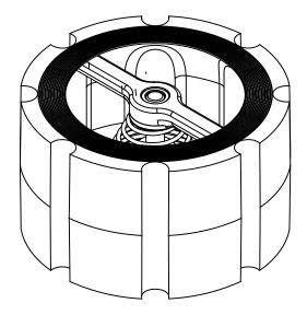
Max Temp 200°F (93°C) Max Inlet Pressure @ 150° F (65°C) 150# 300 psi (21bar) Max Inlet Pressure @ 150° F (65°C) 300# 500 psi (34bar)
