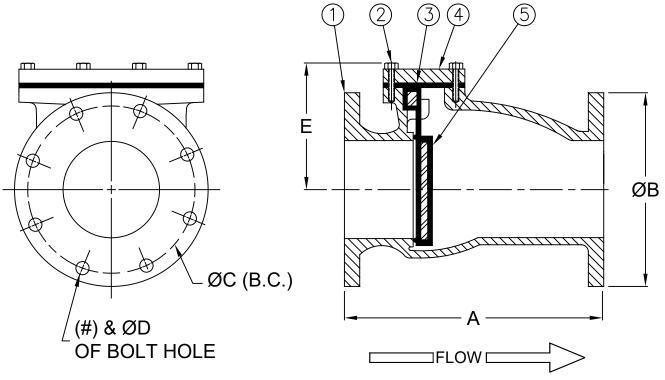
Max Temp 140°F (60°C) Max Pressure 200psi (14bar)
