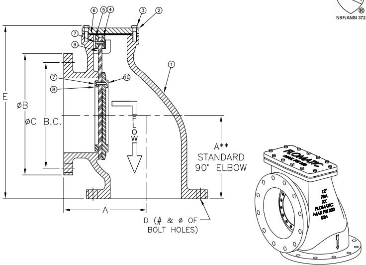
Max Temp 140°F (60°C) Max Inlet Pressure 200psi (14bar)
