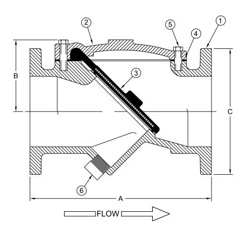
Max Temp 140°F (60°C) Max Pressure 250psi (18bar)
