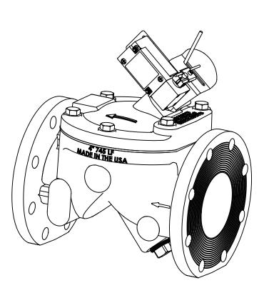
Max Temp 140°F (60°C) Max Pressure 250psi (18bar)
