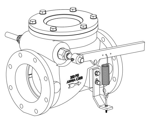
Max Temp 180°F (82°C) Max Pressure 250psi (18bar)
