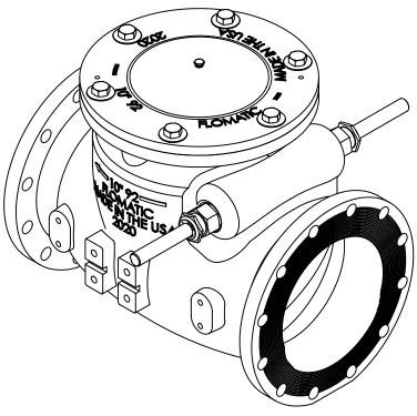
Max Temp 180°F (82°C) Max Pressure 250psi (18bar)
