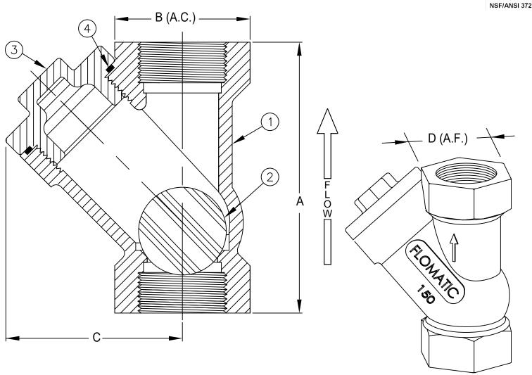
Max Temp 180°F (82°C) Max Inlet Pressure 150 psi (10 bar)
