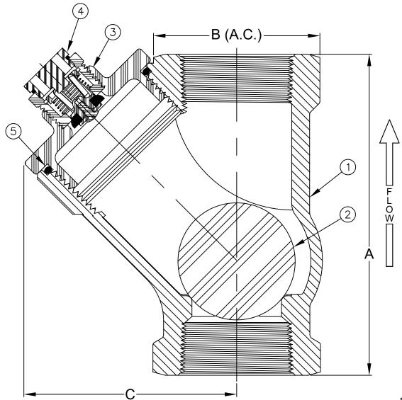
Max Temp 180°F (82°C) Max Inlet Pressure 150 psi (10 bar)
